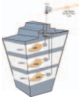
Figure 2 – Using High Speed PtP Wireless to Provide High Speed Access Links to MBU sites
