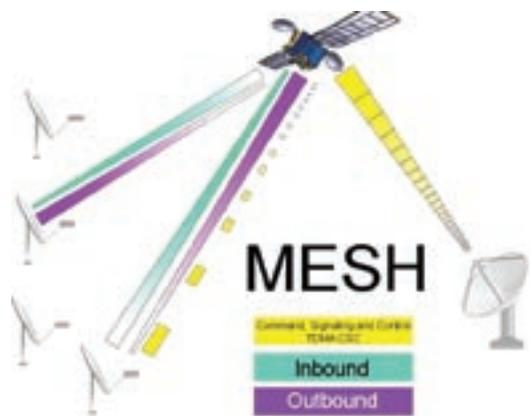
The SCPC mesh/DAMA system works differently. This time a VSAT uses a TDMA CSC (command, signaling and control) channel to request the hub to set up a link from the requesting VSAT and another VSAT. The hub then informs the called VSAT of the request and allocates two channels to serve as a bi-directional link between the two VSAT sites. After the data has been exchanged, the call is finished and the channels are returned to the pool for the next request. Much like a dial up network.
