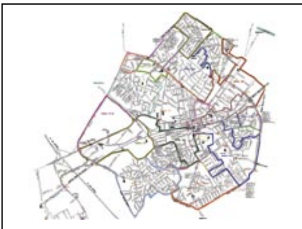
Left: City map of Manassas showing how the city has been divided into several “BPL areas” to assist with network planning. Right: Map of BPL area 303 (it is southernmost area on city map). Orange line indicates the E-PON fiber route, red circles indicate the HFBPL node locations (where E-PON meets the BPL). Blue lines indicate BPL network operating over the existing power grid.
