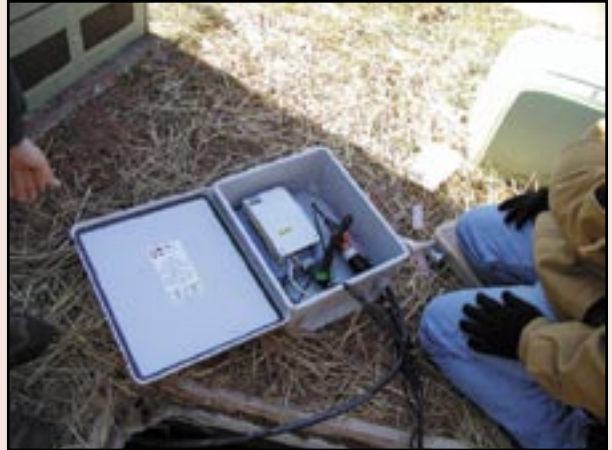
A typical fiber-to-powerline conversion point, installed in a pad-mounted transformer (left) and the E-PON Optical Network Unit (ONU) opened to see the inner workings (right). Each node location services anywhere from 10 to 40 customers with BPL service.
