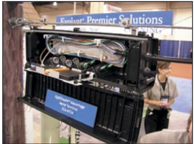
Inside Corning's OptiSheath aerial terminal.
