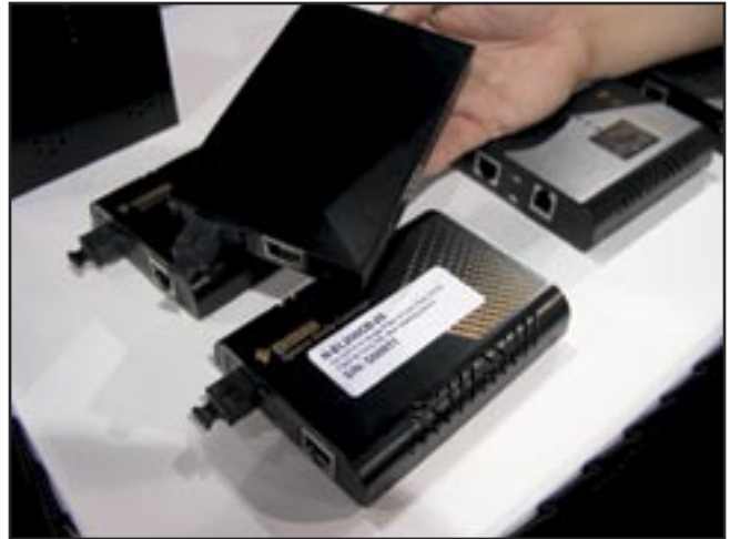
EtherWan optical-to-Cat-5 Ethernet ONT for indoor use; there are several versions of this compact design.
