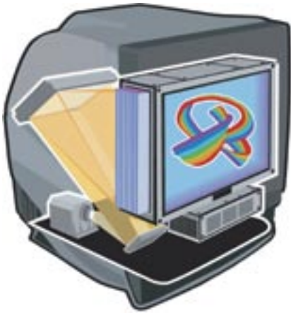
Figure 2 – Volumetric display available today. Source: LightSpace Technologies.
