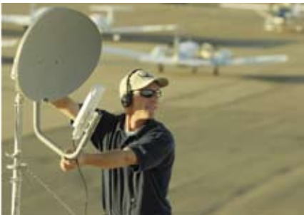
Figure 5. A small dish can be added to the subscriber module for locations more than 5 miles from a WiMAX base station.
