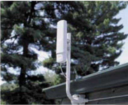
Figure 4. Subscriber module, if the home is not farther than about 5 miles from a WiMAX base station.
