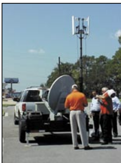
Figure 3: Lightweight trailer carrying a WiFi access point—complete with backhaul antenna and its own gasoline generator.
