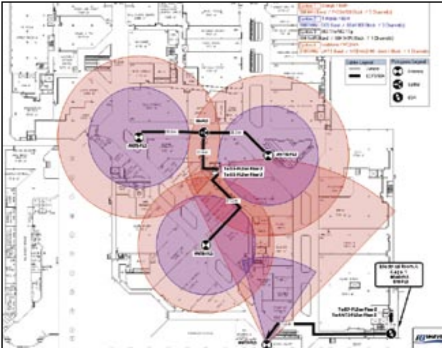
Property owners and installers can use the free RF-vu Viewer to review engineers' designs. Engineers, operators and integrators can collaborate using the Designer Pro version of RF-vu.
