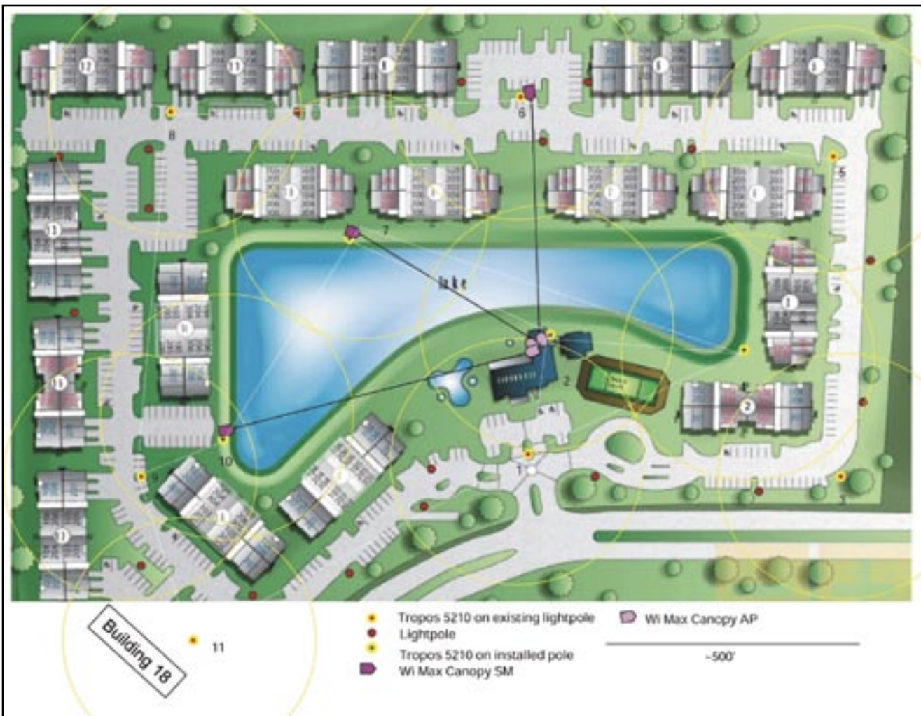
Typical design of an MDU WiFi network.
