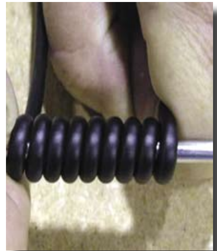
Figure 5. Corning nanoStructures-based fiber in tight bends with no performance impact.
