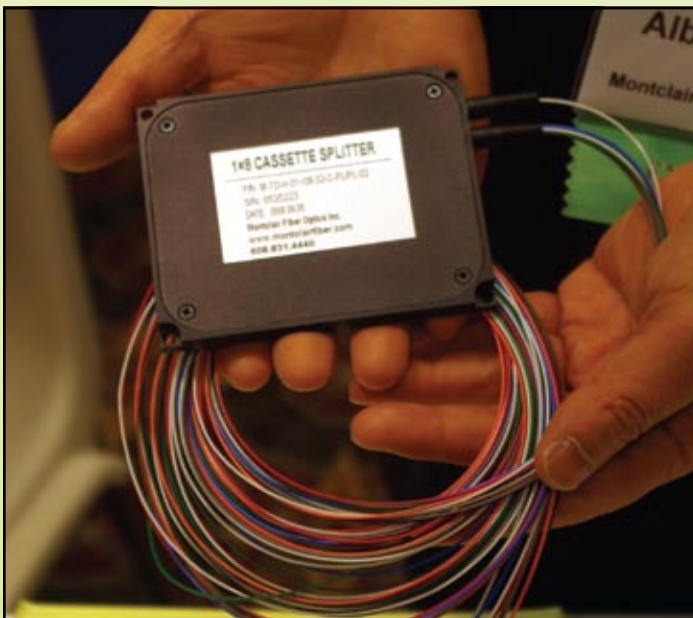
This tiny 1x8 cassette splitter from Montclair Fiber Optics finds its way into FTTB and FTTH inside and outside plant.
