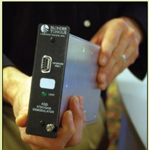
Active electronics are also getting smaller. This ATSC/QAM demodulator is from Blonder Tongue.
