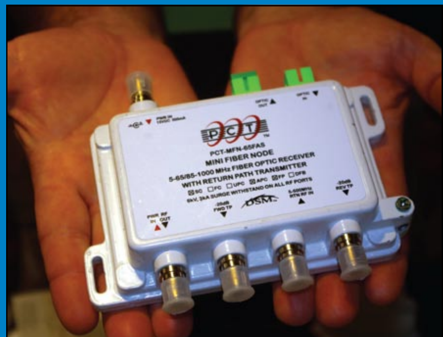
Full-function optical mini-nodes like these can be mounted almost anywhere in an MDU.
