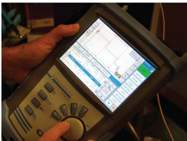
Modular OTDR from EXFO is handheld but heavy (about 6 pounds). This device has two module bays, for handling a wide variety of tasks.
