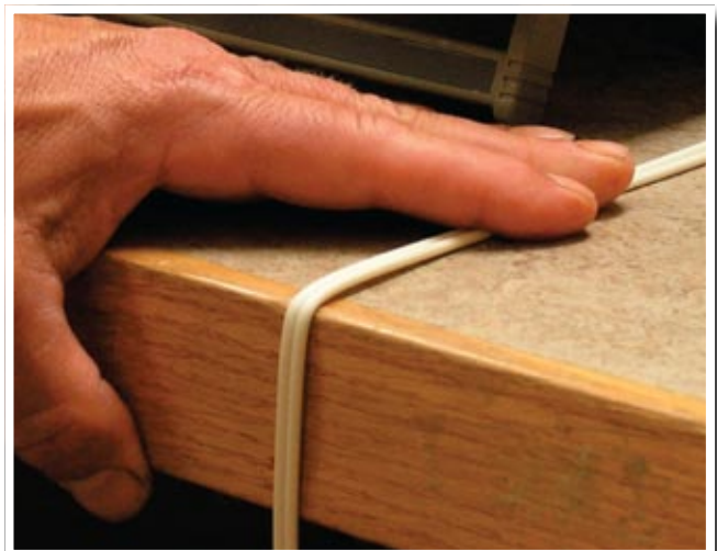
Figure 3. A for-test-only zipcord with a bend-optimized fiber and a standard ESMF fiber, bent around a single sharp corner. The measured loss was 5.45 dB for the ESMF fiber and only 0.01 dB for the bend-optimized fiber at 1550 nm.
